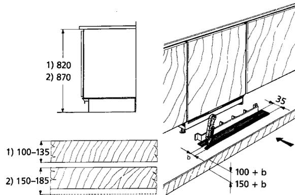
Variant C: Continuous plinth strip cut out, ventilation grid shortened
