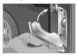
The replacement bulb must be resistant to temperatures up to 300 °C. You can order one from Technical Service.
