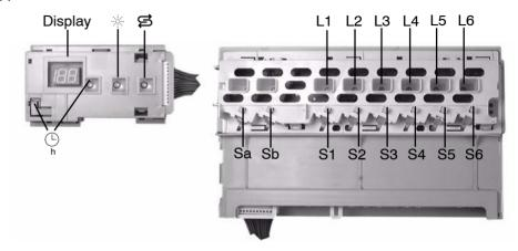
If neither of the two special function buttons (Sa/Sb) is selected, alternating rinsing has been set. If the soak/top basket special function is selected, the water switch has been positioned for top basket. If the time reduction/bottom basket special function is selected, the water switch has been positioned for bottom basket.
