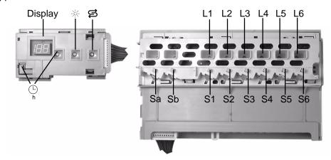
If neither of the two special function buttons (Sa/Sb) is selected, alternating rinsing has been set. If the soak/top basket special function is selected, the water switch has been positioned for top basket. If the time reduction/bottom basket special function is selected, the water switch has been positioned for bottom basket.
