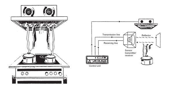
An ultrasonic sensor measures the change in the air density. This change can be caused by:
