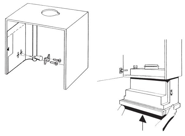
For dismantling, undo one fastening screw until the cooking hood drops on this side and holds itself in an inclined position. Undo the fastening screw on the opposite side until the screw head rises slightly. The bracket of the fastening element remains clamped by a groove on the rear edge and the cooking hood does not fall down. **Note:** While the two fastening elements are undone, do not exert any upward pressure from underneath.
