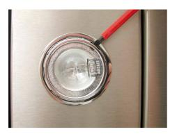
In order to replace the halogen lamps (2x 20 W, Type G4), clip out the glass cover with a screw driver and remove the halogen lamp from the plug base.
