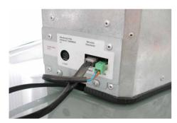
Remove the two group sockets and the two screws.
