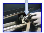
• Remove the upper front panel and check if the connector is inserted properly.
