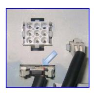
Disconnect the connectors one by one, paying special care in reconnecting them properly in the new board.
