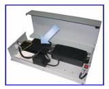
Check if 12V are in the electro-mechanic transformer secondary.
