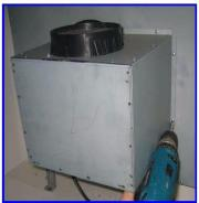
• In case of external motor version (EM) remove the air-outlet flange.
