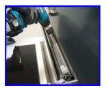
Check if wires inside the neon tube holders contacts are inserted properly.
