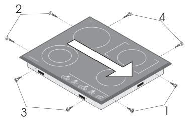
By skilfully tightening the screws (one screw, then the screw on the opposite side and so on) you can slightly adjust the position of the marked cooking zones on the glass ceramic top in relation to the heating spirals.
