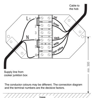
Two-phase connection 400 V system with 230 V phase against neutral conductor
