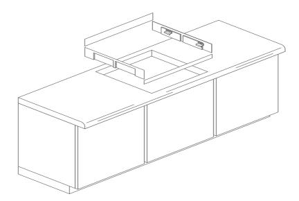
d) Secure support angles on the left and right in the switch panel recess with the enclosed screws in such a way that there is a distance of 502 mm between the notch points (see Fig.).
