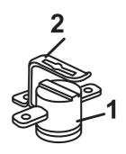
After removing the appliance rear panel, the temperature protection fuse (1) is accessible at the top right of the oven chassis rear.
