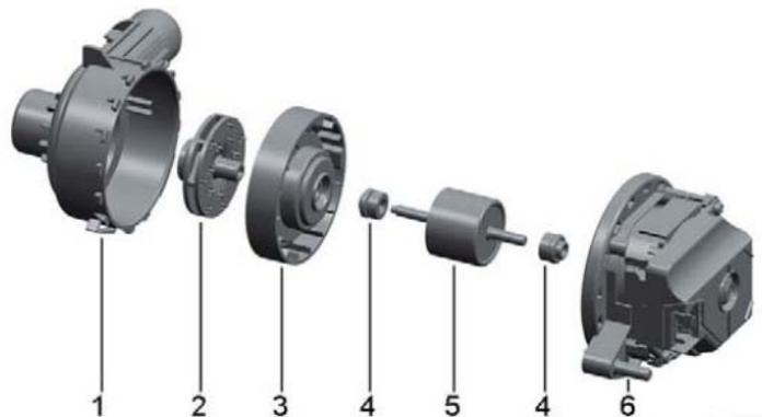
The motor does not have any thermal winding protection since the motor electronics unit detects faults and overloading automatically and switches the motor off.
