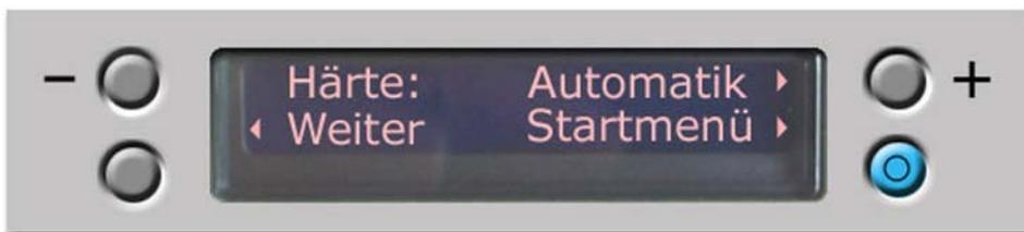
For the manual setting the hardness range can be setting at 8 different levels with the +/- buttons.
