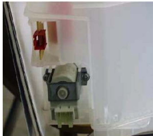
Water softener with a regeneration dispenser.
