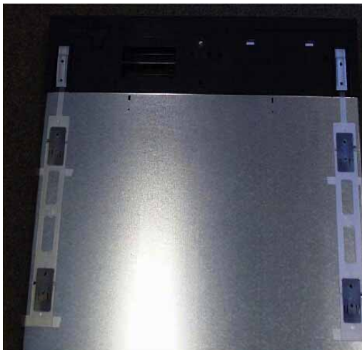
Elements for fixing the wooden door onto the outer door
