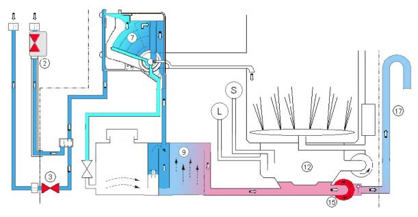
During this phase, the two functions (fill and drain) are performed simultaneously.
