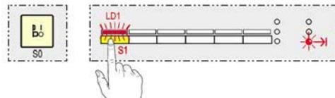
5. Press button S1 for the fourth time: the system proceeds to the activation of the various actuators.
