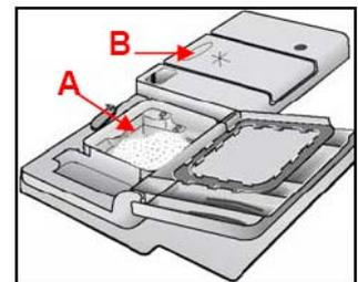
The coil of the detergent dispenser (DD) is powered by the circuit board via triac TY5 (connector D7) at certain points during the cycle, thus ensuring correct dosage.
