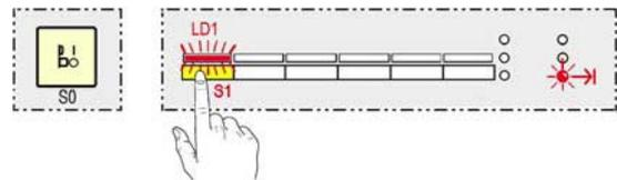
6. To store this setting in memory: press button S0 to switch the appliance off, or wait for 60 seconds (LD1 - LD6 light).
