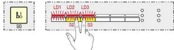
Example: If the current regeneration level is 5, the end of cycle LED will flash 5 times, accompanied by 5 “beeps” from the buzzer. The sequences of flashes and buzzes are separated by a short pause.
