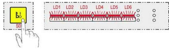
4. Press button S1: LEDs LD2 and LD3 switch off, while LD1 continues to flash. The end of cycle LED begins to flash in synchronization with the signal from the buzzer, indicating the level of regeneration
