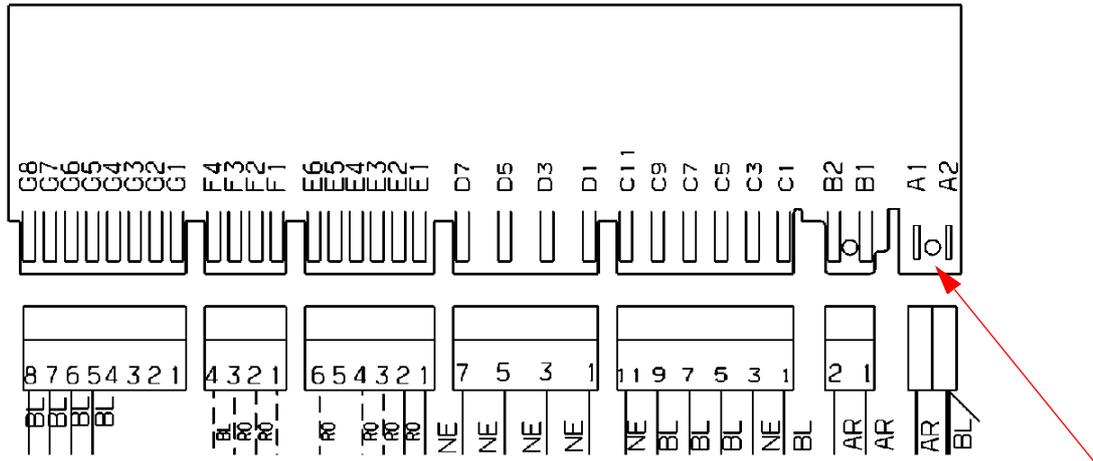
**Caution!** Care should be taken relative to the position of connector “A1 - A2”: if this connector is replaced in the incorrect position (back-to-front), the appliance will *not function*. The board will not accept any commands since the power supply will be disconnected.
