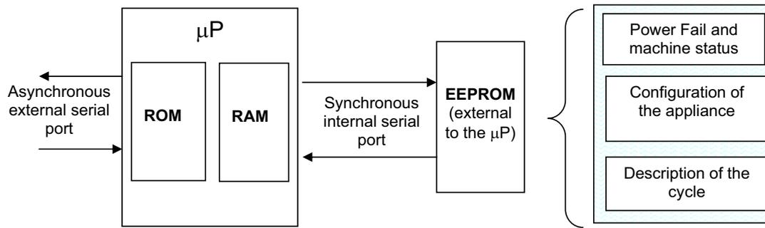
The main circuit board features an EEPROM memory (external to the microprocessor) which stores in memory data relative to the configuration, description of the cycle, cycle status in case of a power failure, and any alarm conditions. The configuration data (entered in the factory using a computer with a DAAS interface) determine the functionalities of the appliance (number and type of programmes, options, LEDs etc.).
