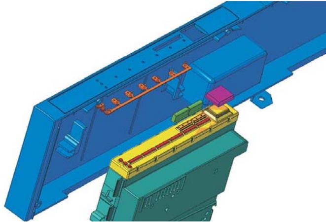
The EDW 503 control system consists of a main circuit board and a control/display board. Both boards are housed in a plastic container (fig. 1). The On/Off function is performed by the button S0.
