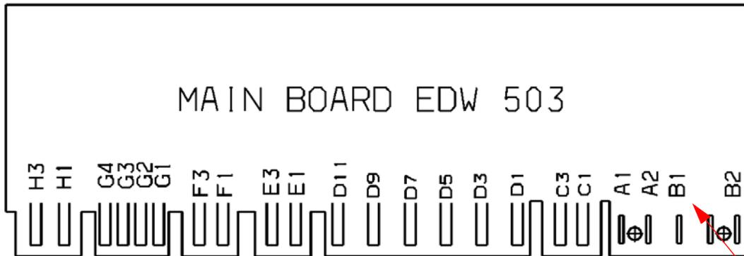
**Note:** Care should be taken relative to the position of connector “B1” - “B2”: if this connector is replaced in the incorrect position (back-to-front), the appliance will *not function* since the power supply will be disconnected.
