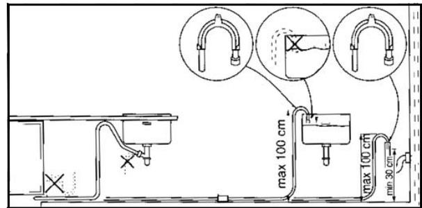
Thus, if alarm iF0 occurs, it is a good idea to make sure the drain tube is correctly positioned as shown in the instruction manual.
