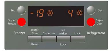
The coldest temperature setting is selected with the Super Freeze button.
