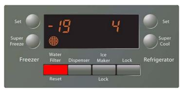
Replace water filter display: press the Water Filter reset button for three seconds in order to reset the display.
