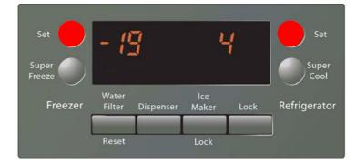
The temperature of the freezer compartment is set with the left-hand button for making settings.
