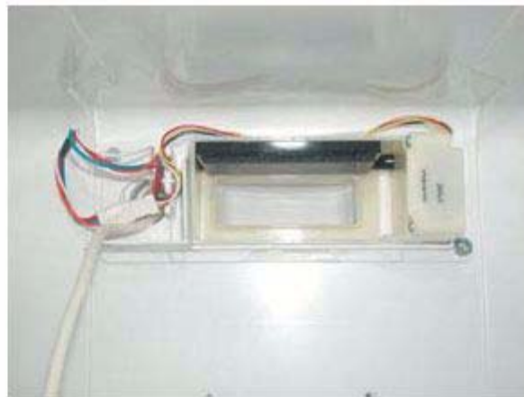
6. The damper is fastened with 2 screws; it is connected to the electric wiring with a 4-pole connector.
