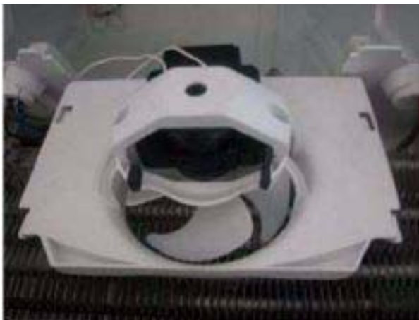
11. The fan is fastened to the holder which pulls out of the evaporator module.
