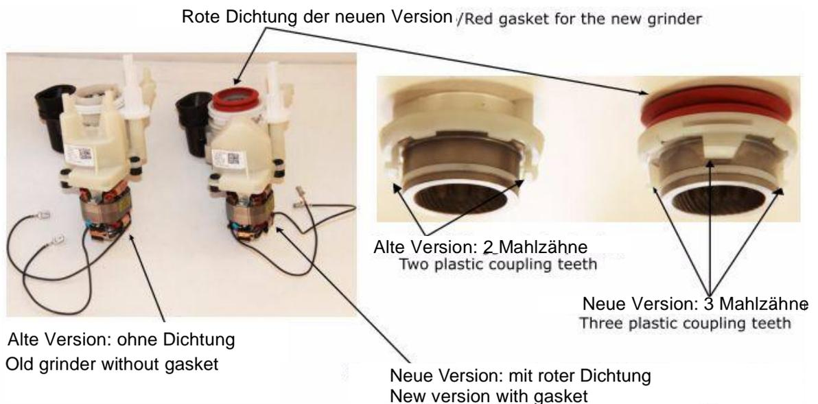
*We inform you that, since March of 2013, a new grinder is fitted in the model EKV6500.1, series number SN 273074 AP 13032080001. As you can observe in the pictures attached, new grinder has, among other things, a red gasket in the upper position (noticeable at first sight when the grinder is fitted in the appliance), absent from the previous one, besides three plastic coupling teeth (instead of two of the previous version) used to assembly the external mill to the grinder.*
