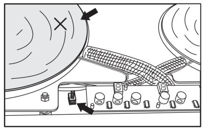
Unplug and pull sensor cable out under the sheet metal.
