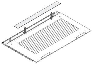
Take the protective foil off the metal strip and glue it in place between the two fastening screw holes of the door handle on the inner side of the front pane.
