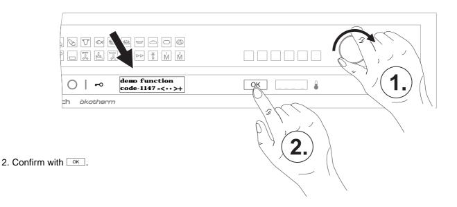
1. Turn the knob clockwise to activate the demonstration mode or counterclockwise to disactivate it.
