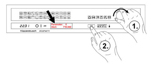
Turn the dial knob until the display shows SETTING: 716.000 and then confirm by pressing OK.
