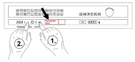
First of all press the button for the child safety lock and then immediately press the concealed "set clock" button, located between the clock and the "0" off button, for a little longer. The display will show: PARAMETER: 0 and SETTING: 0.00.
