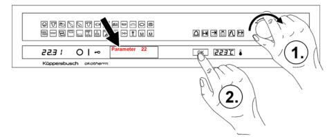
Turn the dial knob until the display indicates PARAMETER: 22 and press OK to confirm. The display will show: PARAMETER: 22 GeType and SETTING: 6810.00 (or another setting).
