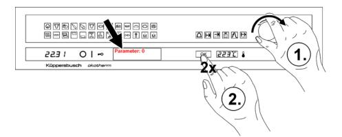
Turn the dial knob until the display shows PARAMETER: 0 and press OK twice to confirm.
