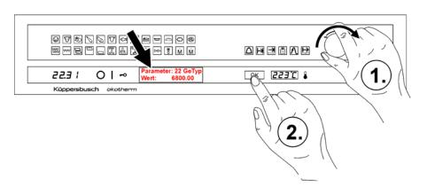
Turn the dial knob until the display shows SETTING: 6800.00 and press OK to confirm.
