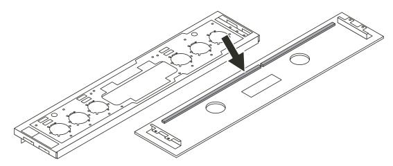
2. Glue new foam sealing material into the groove along the contour of the metal panel as illustrated.
