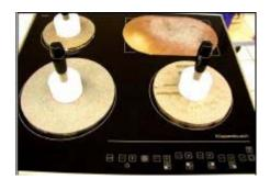
If calibration has been completed successfully for all the cooking zones, the controls will automatically switch off the calibration process. The alarm buzzer will sound and the controls will switch to normal operation, i.e. the touch control is OFF and is waiting to be switched on with the main switch.
