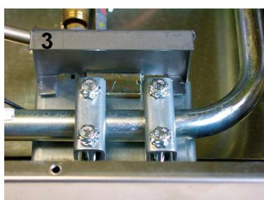
4. For the GWS 457.0 WOK two service kits are used and are positioned with the surfaces (as indicated under 3) on the two support sheets. The upper surfaces (3) of the supporting sheets support themselves on the inside of the base once it has been screwed on.
