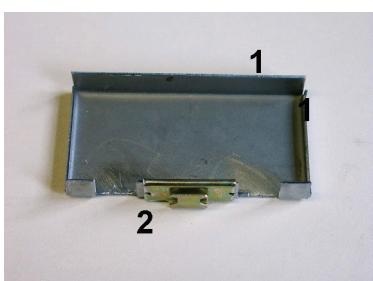
2. The service kit comprises a supporting sheet (1) and inserted spring (2). For GKS 300 WOK (produced before September 2003) the service kit with an overall height of 54.5 mm is to be used and for all of the other models the service kit with an overall height of 39.5 mm is applied.
