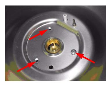
Loosen the three burner fastening screws by a quarter to a half rotation after they have been fastened.
