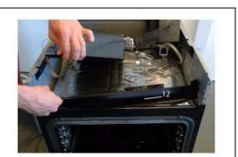
8. IOnce it has been removed, the "old" cross bar can be compared to the "new" one.
