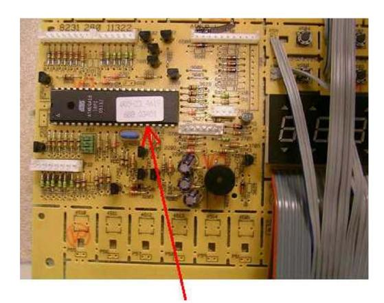
In this example the production date of the printed circuit board is W05-23 (05 = year, 23 = CW 23)
