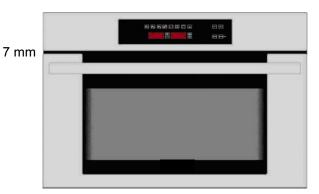
The door can also be aligned when it has been mounted. The hinged door holder (spare-part no. 528895) must be released in order to relieve the door tension. The door will then need to be adjusted so that the clearance between the door and the control panel is 7 mm. The screws are then tightened again.
