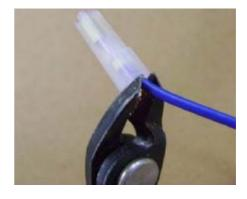
**5.** Cut approx. 5 mm off the sheath and expose the wires.
