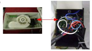
2. Disconnect the 4 wires from the green resistor.
