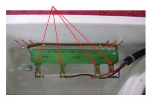
**3.** Remove all the green resistor wiring.
