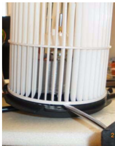
Figure 8: Make sure there is not turbine vs motor base interference before placing it back.
