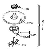
• The old components labelled 116, 132A and 120B **cannot** be replaced individually by the new ones but **only in total**.
