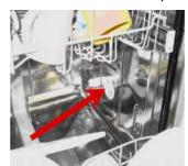
7. An additional possibility to prevent damages on the kitchen furniture after a longer time is to seal the holes of the topbox from the drying system to the tub by using an appropriate silicon or by installing a new 2 mm-thick seal.
