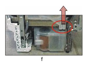
Note! When re-mounting, lubricate the O rings and fit them exactly. Make sure that the flow in the hose is not blocked off anywhere between the pan itself and the side panel.
