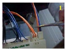
4. Strip the wires just long enough for the correct insertion into the tag.
