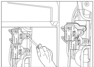
Loosen the defrost thermostat switch (upper thermostat).
