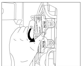
Bend the fitting plate, on which the defrost thermostat switch is mounted, slightly forward so that the thermostat switches are not in the direct air current of the filament resistance of the evaporator.
