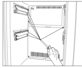
Loosen the screws and remove the two guide rails on one side.
