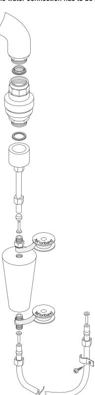
Appliance connection valve with integrated return valve (customer-provided)
