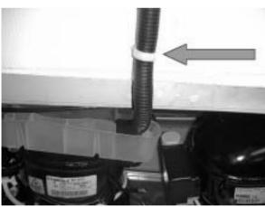
Fix the bottom part of the drain tube with a fastening clamp and make sure the tube is placed in the water basin correctly.
