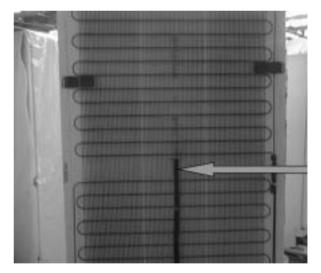
Reposition the condenser and fasten it with the 4 screws.
