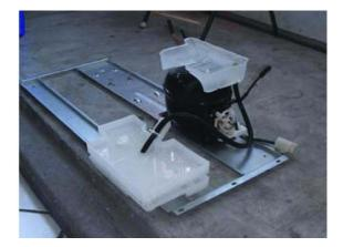
5. Cut off the protruding part of the hose and fasten it to the drip collecting tray with a hose strap.
