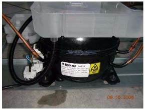
4. The water discharge hose is guided behind the compressor, as shown on the illustration.
