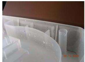
2. Cut a notch into the discharge pipe of the vapour tray located on the compressor as shown on the illustration.
