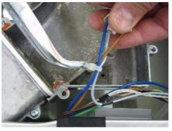
CAUTION! It is essential to seal the edge of the heating element with a suitable adhesive before installing the element. Replace the cable in the slot.
