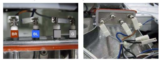
Remove the black "jumper". To do so, first of all cut off the faston connector.
