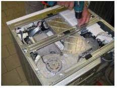
3. Remove the screws from the dryer cover.
