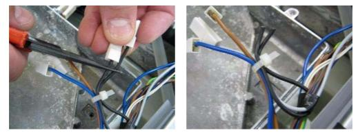
Then remove the cable and tighten the cable clamp.
