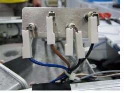
5. Replace the heating element with the new heating element.
