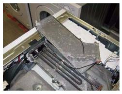
4. Remove the two fastening screws from the heating element.
