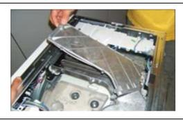
4. Lift and remove the heating element cover.
