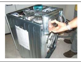
2. Use a crosshead screwdriver to remove the 6 screws in the rear crosspiece, then set them aside.
