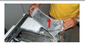
5. WARNING! During reassembly, make sure the gasket is positioned correctly.
