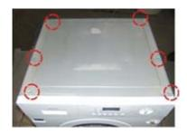
1. Remove the top, which is fixed to the appliance by 6 screws.
