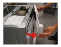
3. Pull the front panel outwards, disconnect the wires and ...
