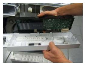
6. ... the timer, which is fitted into the front panel, and replace it with the new timer updated.
