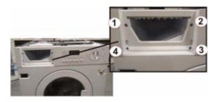
2. Remove the detergent drawer and unscrew the 4 screws indicated securing the gront panel.
