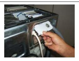
Remove the water inlet hose and remove the plastic solenoid valve cover on the rear crosspiece.
