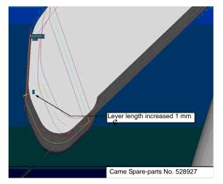
Replace Inner Door Frame for a new version Thickness increased 1mm and base reinforced.
