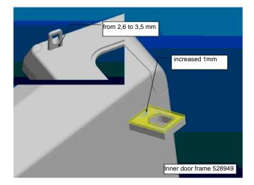
With these improvements we assure an adequate mechanical action on the came resulting a good working stability. Extreme working positions will be controlled by the hook without the possibility of came returning to the safety position after hook freedom.
