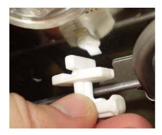
New ceramic holder after insertion in the special shaped hole and 90° rotation.
